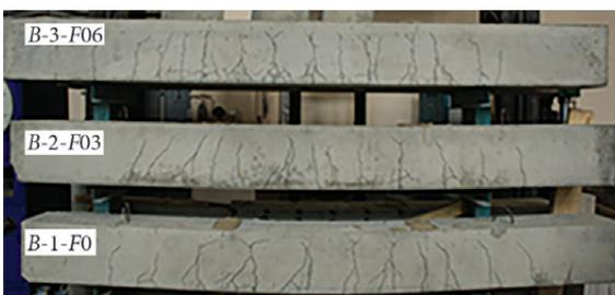
**Fig. 8.** The final crack pattern of the full-scale beams
