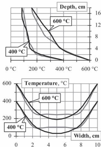
**Fig 10.** Experimental (grey curve) and calculated (black curve) temperature distribution along (above) and across section (below) of the beams exposed to 400 °C and 600 °C
