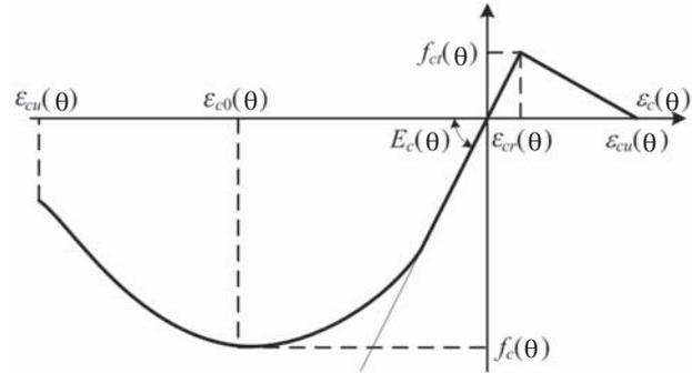
Fig 4. Model of stress-strain relationship of concrete
