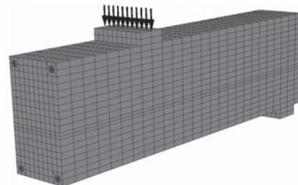
Fig 8. The finite element model used in numerical analysis by software MSC.Marc
