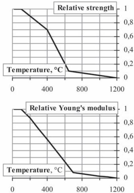
Fig 7. Reduction of strength and Young's modulus of steel at elevated temperatures
