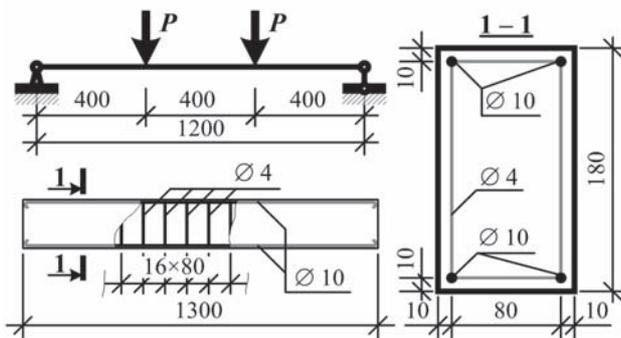
Fig 2. The loading configurations and specimen dimensions
