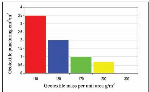
Fig 7. The total area of geotextile punctures cm<sup>2</sup> per m<sup>2</sup> in the second test section
