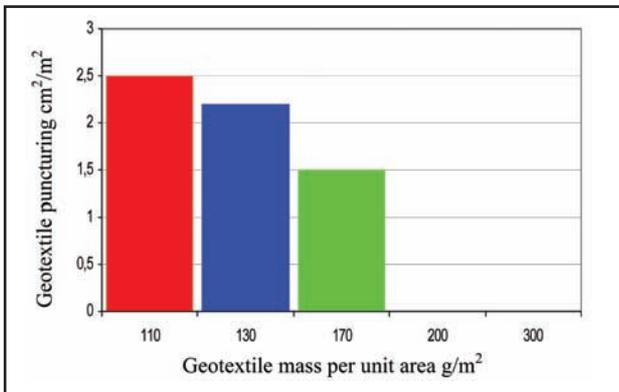
Fig 6. The total area of geotextile punctures cm<sup>2</sup> per m<sup>2</sup> in the first test section
