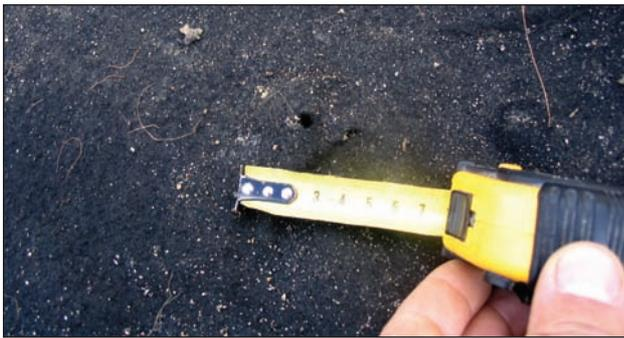
Fig 4. Samples of geotextile damages (puncturing) whose mass per unit area is 110 g/m<sup>2</sup> laid between the subgrade and the frost blanket course
