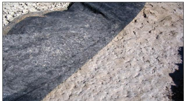
Fig 9. The performance of the road pavement layer separation by geotextile after uncovering the layers of the second test section of the pavement structure – the separation of the frost blanket course and the sub-base
