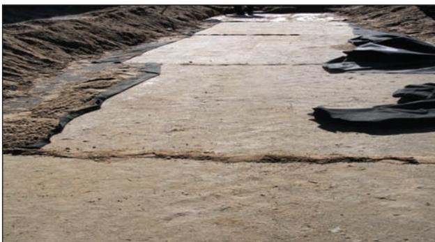
Fig 8. The performance of the road pavement layer separation by geotextile after uncovering the layers of the first test section of the pavement structure – the separation of the subgrade and the frost blanket course
