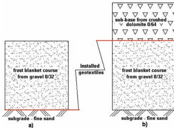
**Fig 3.** The levels of geotextile installation: a) geotextile separating the subgrade and the frost blanket course, b) geotextile separating the frost blanket course and the sub-base
