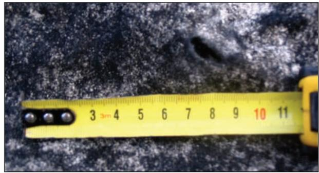
Fig 5. Samples of geotextile damages (puncturing) whose mass per unit area is 130 g/m<sup>2</sup> (laid between the frost blanket course and the sub-base of the pavement)
