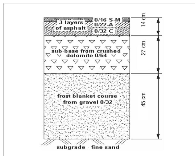
Fig 1. A typical road pavement structure
