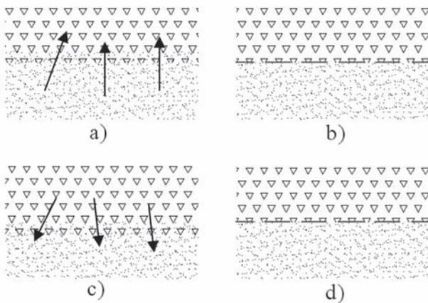
**Fig 2.** Processes active in the layers of the road structure and their prevention by a separation geotextile: a) fine particles of soil migrate into a more porous frost blanket course, b) the migration process of fine soil particles has been terminated, c) large aggregate particles migrate into a weaker layer, d) the migration process of large particles has been terminated
