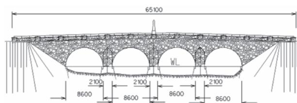
Fig 6. Elevation of stone arch bridge
