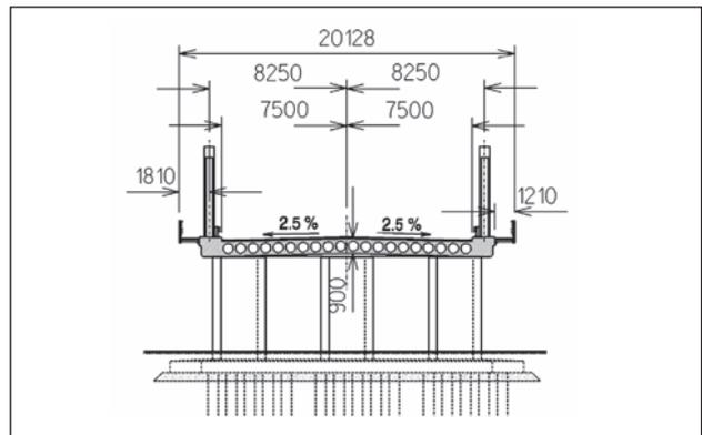
Fig 13. Cross-section of overpass span structure
