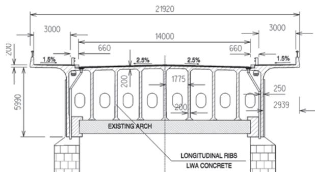
Fig 11. Cross-section of span structure after reconstruction
