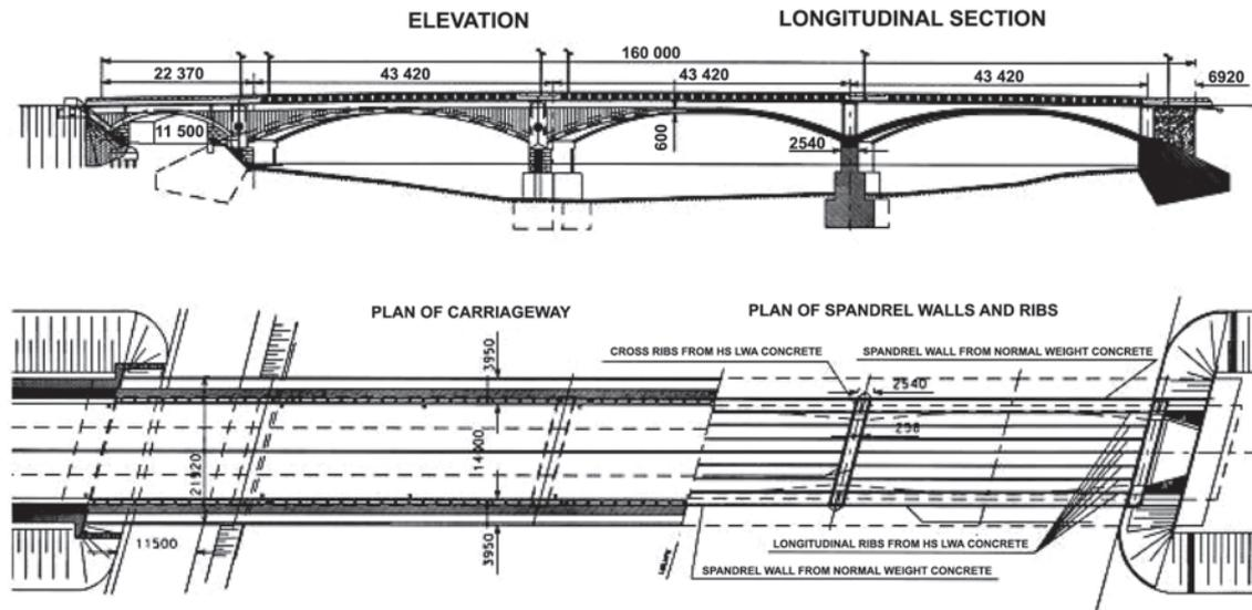
Fig 9. Elevation and section of the bridge structure after reconstruction
