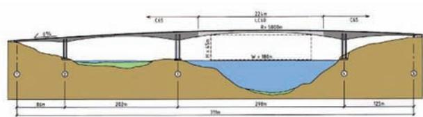
Fig 3. Elevation of Raftsundet bridge in Norway [2]
