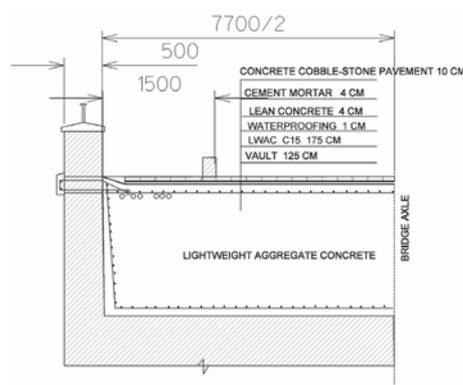
Fig 8. Cross-section of the pier
