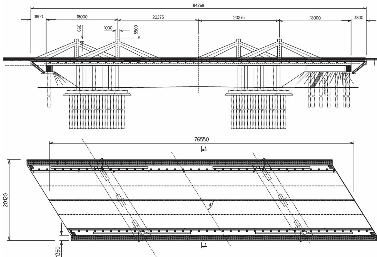
Fig 12. Elevation and plan of overpass
