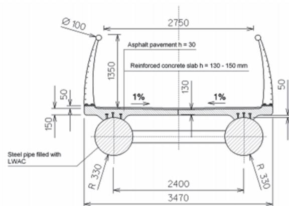
**Fig 15.** Cross-section of the pedestrian bridge
