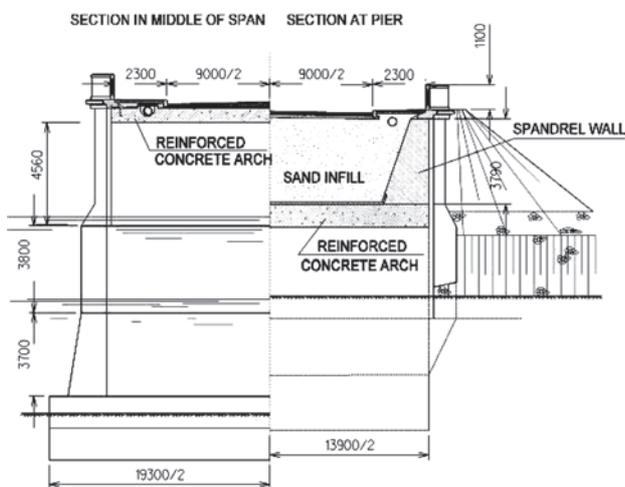
Fig 10. Cross-section of span structure before reconstruction
