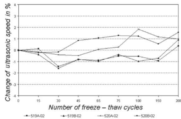
Fig 18. Change of ultrasonic speed depending on the number of freeze-thaw cycles
