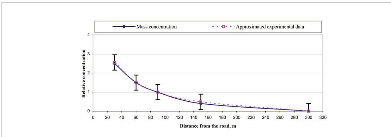
Fig 4. The approximation of total contamination index  $Z_s$  and measured concentrations MC dependence on the distance from the road
