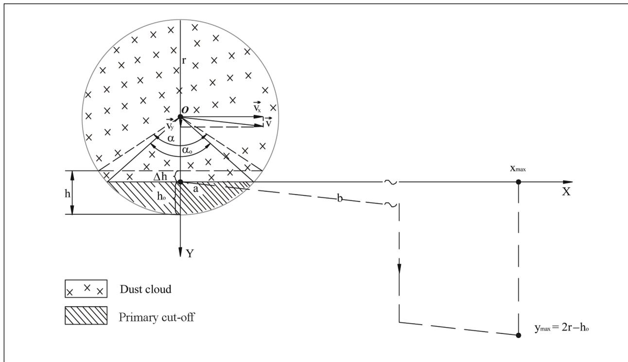
Fig 2. Cylindrical shape whirl of dust with cut-off model
