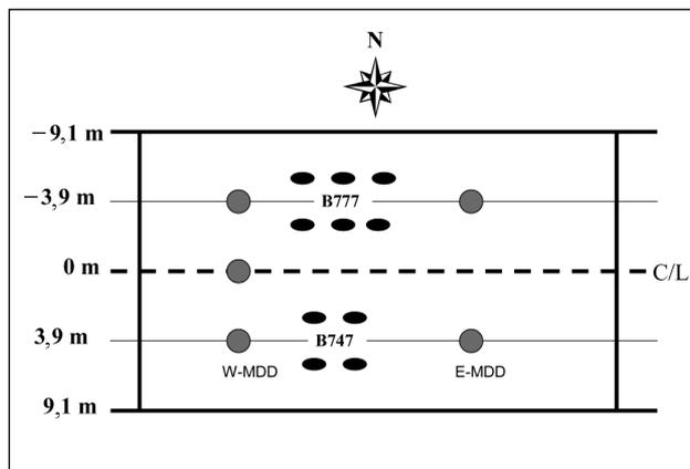
Fig 3. Heavy Weight Deflectometer (HWD) test lane locations
