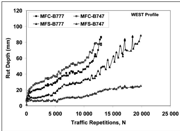
Fig 4. Rut depth progression during traffic testing
