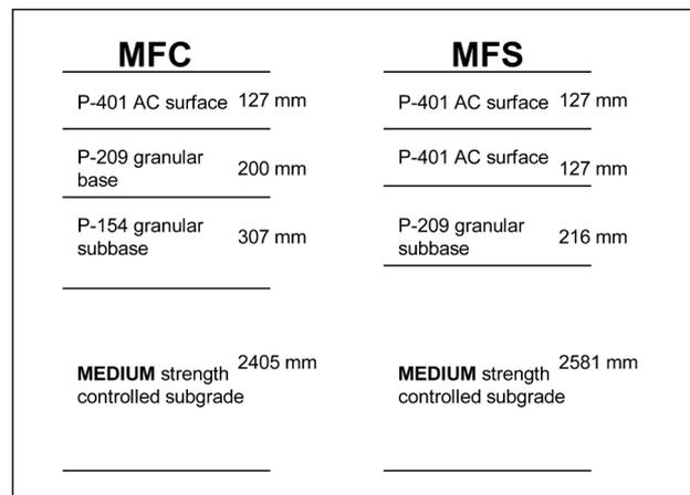
Fig 1. Cross-sectional views of as-constructed NAPTF flexible test sections
