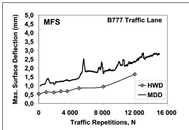
Fig 8. Comparison between HWD and MDD surface deflections in B777 traffic lane (MFS)
