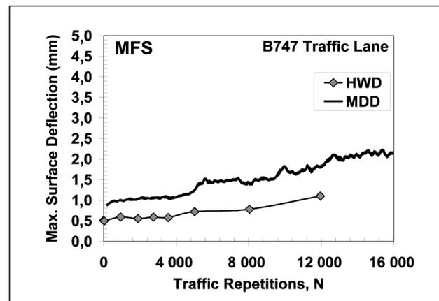
Fig 9. Comparison between HWD and MDD surface deflections in B747 traffic lane (MFS)
