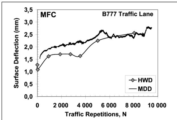
Fig 6. Comparison between HWD and MDD surface deflections in B777 traffic lane (MFC)
