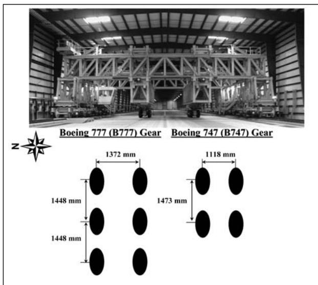
**Fig 2.** NAPTF traffic test vehicle and test gear configuration details
