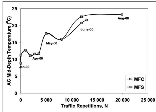
Fig 5. Variation in asphalt concrete mid-depth temperature during traffic testing
