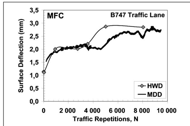
Fig 7. Comparison between HWD and MDD surface deflections in B747 traffic lane (MFC)
