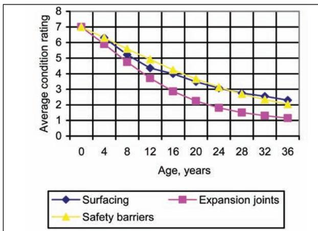
Fig 4. Average condition rating of deck roadway members versus age using Markov model
