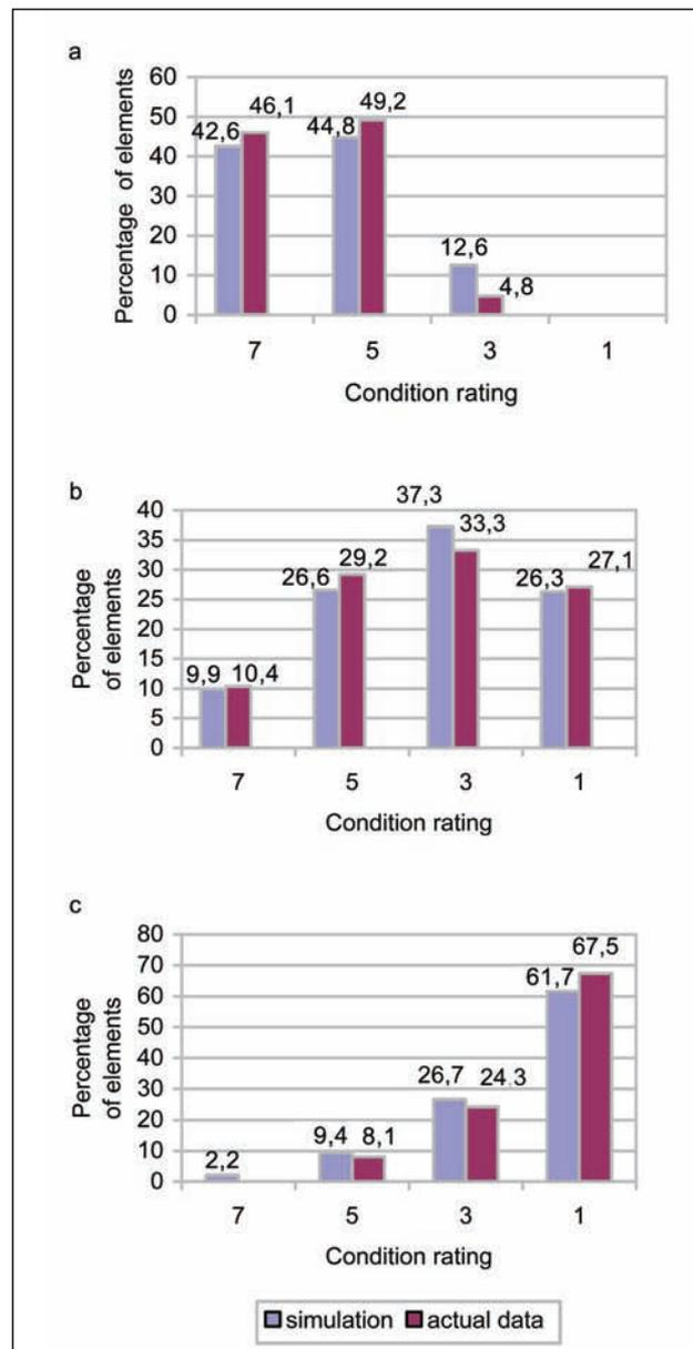
Fig 7. Comparison of observed and simulated condition state distributions of barrier wall elements after 8 (a), 22 (b), and 36 (c) years in service
