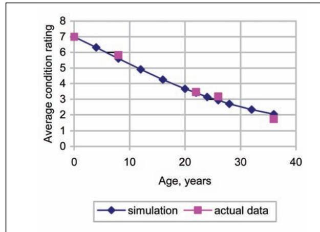
Fig 6. Comparison of Markov simulation and observed safety barriers condition
