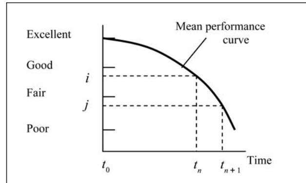
**Fig 2.** Relationship between deterioration of a bridge member and its condition rating
