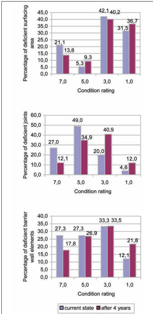
Fig 3. Condition rating of deck roadway members
