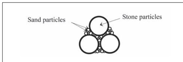
Fig 8. Sand layers reduce interlocking of stone particles
