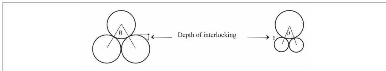
**Fig 2.** Effect of diameter size on  $\theta$  and interlocking depth of spherical aggregate assemblies
