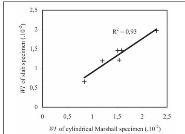
Fig 6. A comparison between  $WI$  values of the Marshall cylindrical specimens and those of the slab specimens
