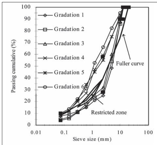
Fig 4. Aggregate gradations used in this research
