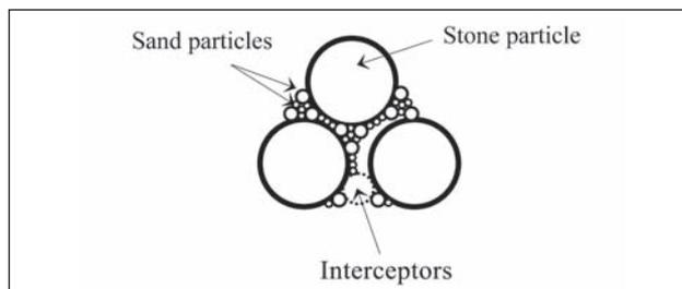
Fig 9. Interceptors reduce aggregates packing
