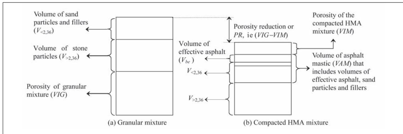
**Fig 1.** Model of aggregates mixture and compacted HMA mixture
