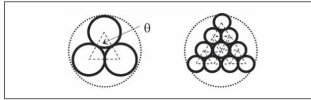
Fig 3. Spherical aggregates assemblies with small and large spherical aggregates occupying the same room
