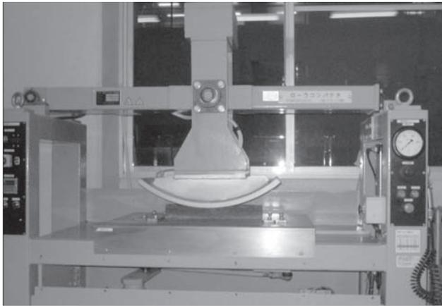
Fig 5. A steel roller compactor
