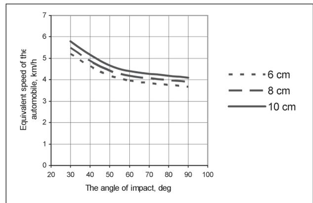
**Fig 10.** Dependence of the minimal automobile speed, equivalent to the expenditures of its kinetic energy at the moment of impact on the road border, when the tire becomes dismantled, on the angle of impact for VW TRANSPORTER
