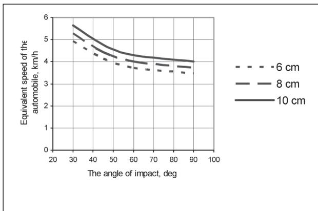
**Fig 9.** Dependence of the minimal automobile speed, equivalent to the expenditures of its kinetic energy at the moment of impact on the road border, when the tire becomes dismantled, on the angle of impact for MAZDA 626
