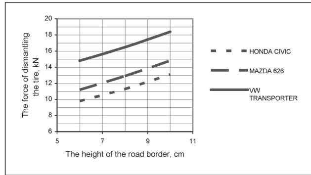
Fig 3. The minimal force, necessary for dismantling the tire from the rim
