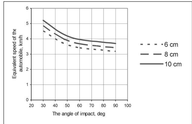
**Fig 8.** Dependence of the minimal automobile speed, equivalent to the expenditures of its kinetic energy at the moment of impact on the road border, when the tire becomes dismantled, on the angle of impact for HONDA CIVIC
