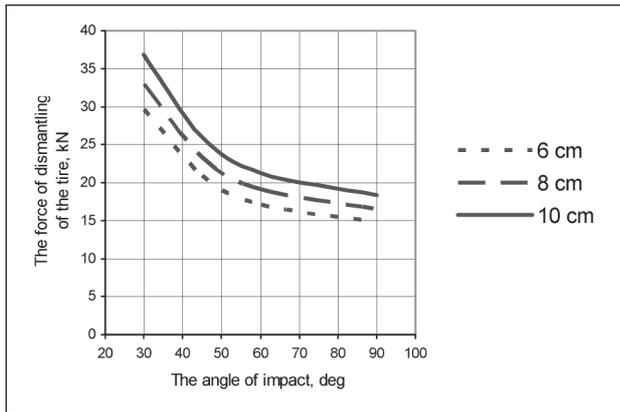
**Fig 7.** Dependence of the force, necessary for dismantling the tire from the rim, on the angle of impact for VW TRANSPORTER
