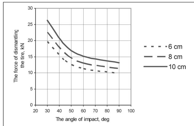
Fig 5. Dependence of the force, necessary for dismantling the tire from the rim, on the angle of impact for HONDA CIVIC
