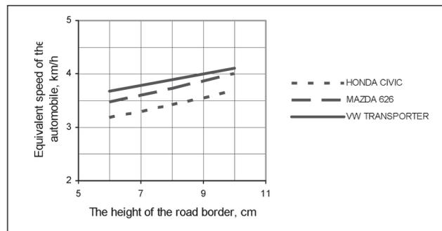
Fig 4. The automobile minimal speed, equivalent to the expenditures of its kinetic energy at the moment of its impact on the road border, when the tire becomes dismantled
