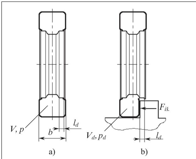
Fig 2. The automobile wheel: a – before the impact on the road border; b – at the moment of impact, just before the tire dismantling
