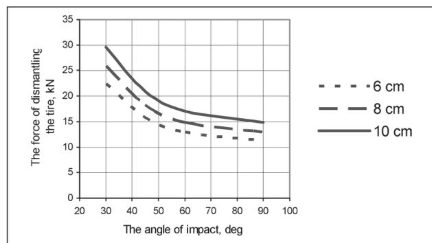
Fig 6. Dependence of the force, necessary for dismantling the tire from the rim, on the angle of impact for MAZDA 626
