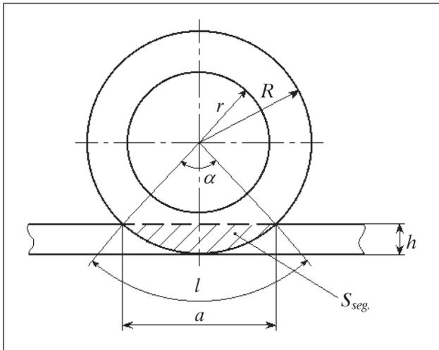
Fig 1. The contact of the side component of the automobile wheel with the road border
