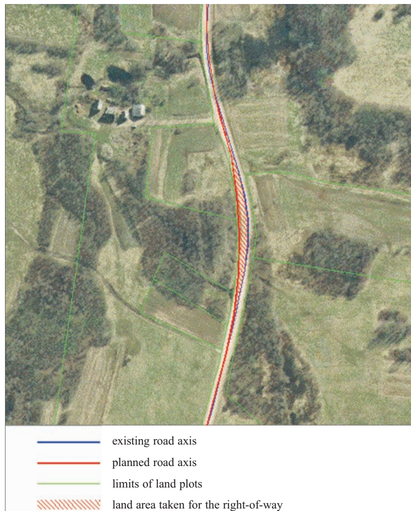
Fig 1. Illustration of the methodology for determining the volume of a possible taking of land for the right-of-way land
