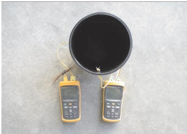
Fig 4. Instrumented 152×305 mm standard cylinder mould
