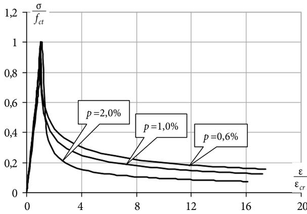
Fig. 6. Numerically derived  $\sigma_t - \epsilon_t$  relationships for varying reinforcement ratio
