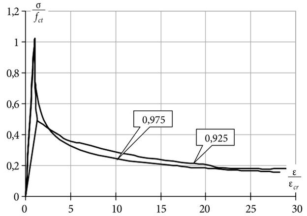
Fig. 8. Numerically derived  $\sigma_t - \epsilon_t$  relationships for varying normalised effective depth,  $d/h$
