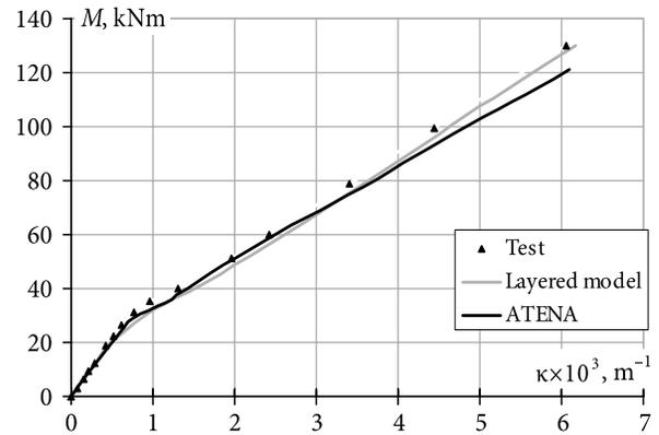
Fig. 9. Experimental and calculated moment-curvature diagrams for the beam 1R
