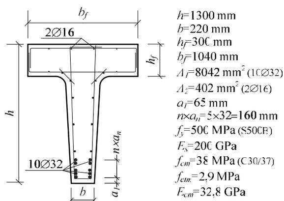
Fig. 11. Cross-section of bridge girder at the mid-span
