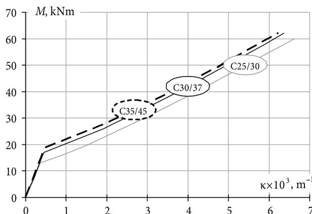
Fig. 4. Moment-curvature diagrams for ranging grade of concrete. Reinforcement ratio  $p = 0,6 \%$
