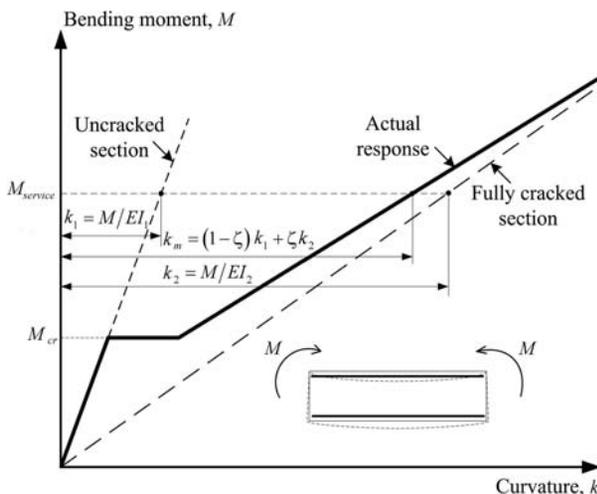
Fig. 1. Moment-curvature relationship according to the *Eurocode 2*
