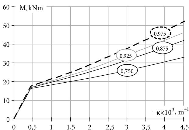
Fig. 5. Moment-curvature diagrams for ranging normalised effective depth,  $d/h$ . Reinforcement ratio  $p = 0,6 \%$ , grade of concrete C30/37
