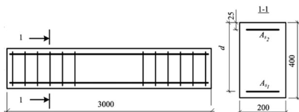
Fig. 2. Details of the beams
