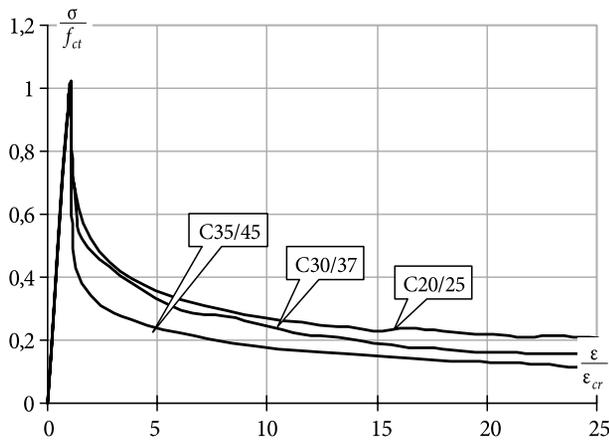
Fig. 7. Numerically derived  $\sigma_t - \epsilon_t$  relationships for varying grade of concrete
