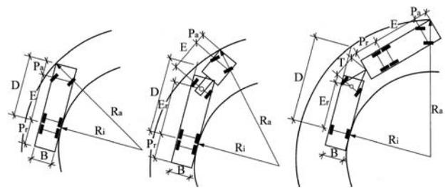
Fig. 6. Reduced wheel base  $D$  for different vehicle type
