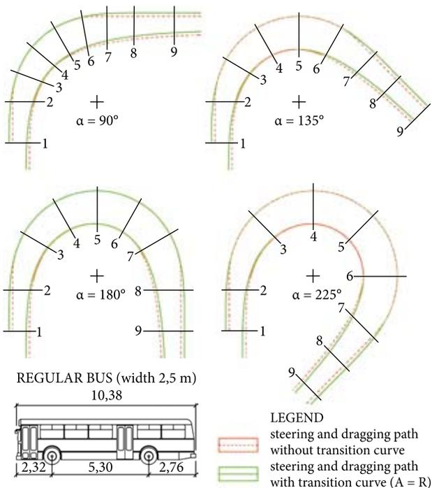
**Fig. 3.** Setting the lane width for different shaping of steering path (turning angle  $\alpha = 90, 135, 180$  and  $225^\circ$ )
