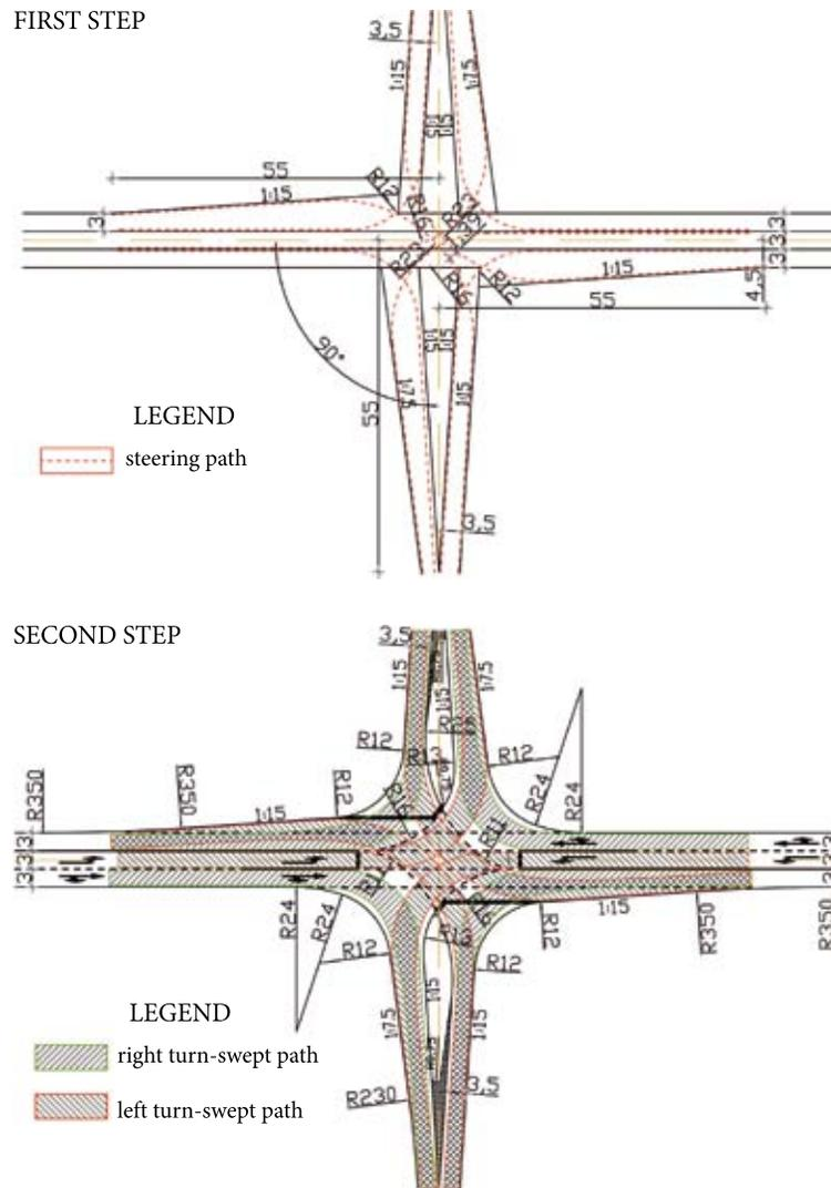
Fig. 9. Four-leg intersection at grade ( $90^\circ$ -angle between main and auxiliary traffic direction)
