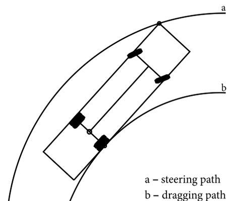
Fig. 1. Vehicle movement trajectories
