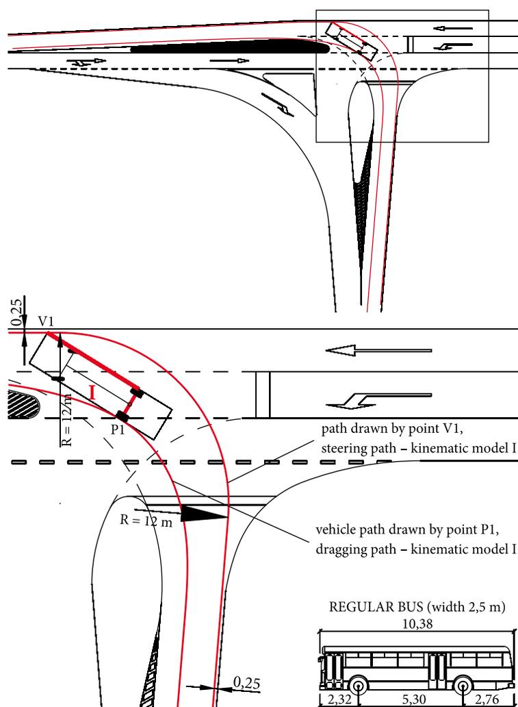
Fig. 4. Setting vehicle movement trajectory – kinematic model I
