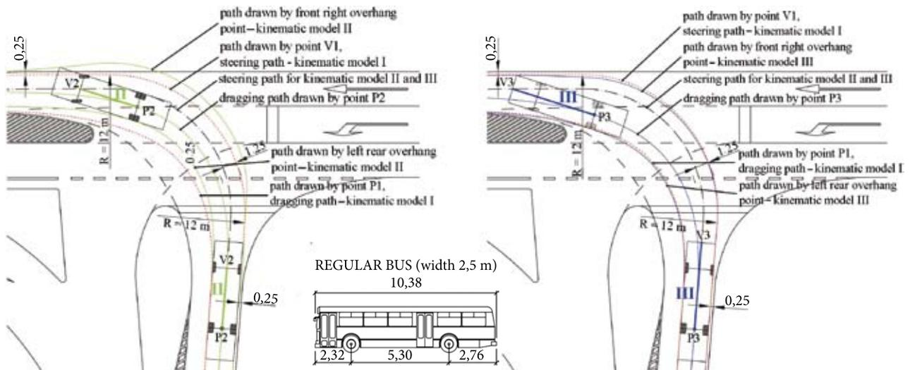
Fig. 5. Setting vehicle movement trajectory – kinematic model II and III
