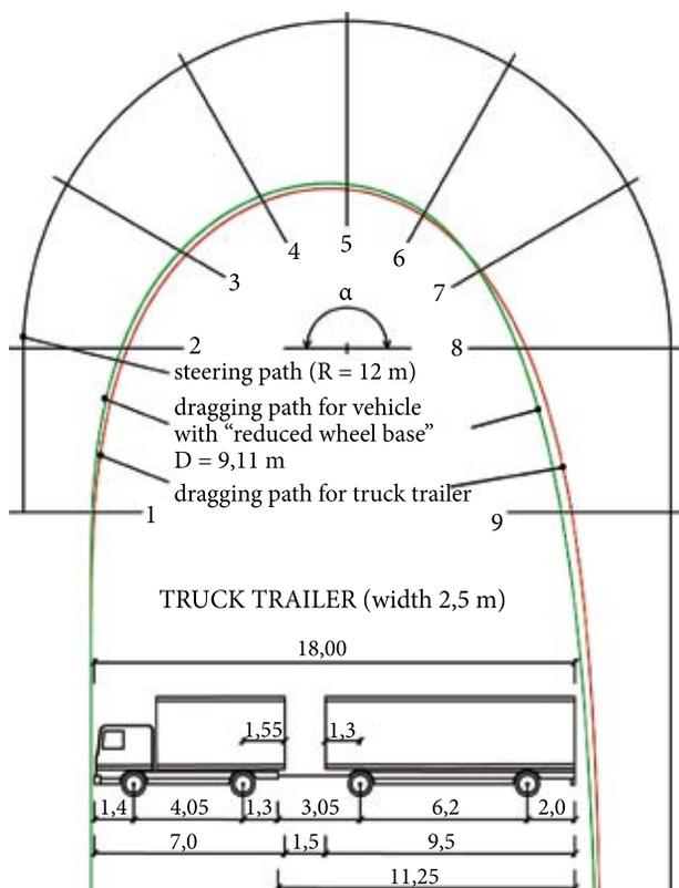
Fig. 7. Setting a complex vehicle movement trajectory (truck semitrailer) by the method of reduced wheel base
