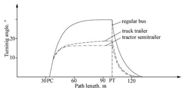
Fig. 2. Theoretical angles of vehicle turning for steering path shaped without transition curves ( $R = 18$  m, turning angle  $210^\circ$ )
