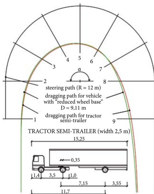
Fig. 8. Setting a complex vehicle movement trajectory (tractor semi-trailer) by the method of reduced wheel base
