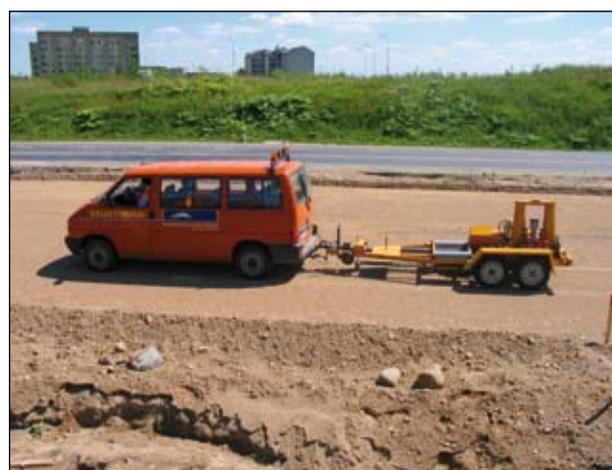
Fig. 4. Falling Weight Deflectometer (FWD)
