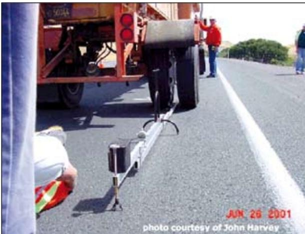
Fig. 2. Benkelman Beam (Washington State Department of Transportation 2006)
