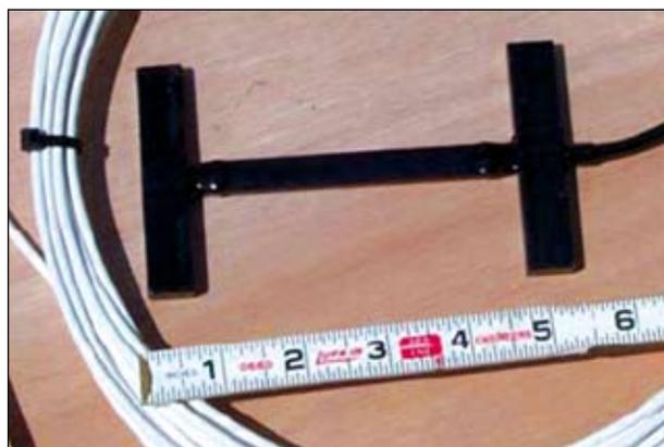
Fig. 2. Strain transducer installed in experimental pavement structures
