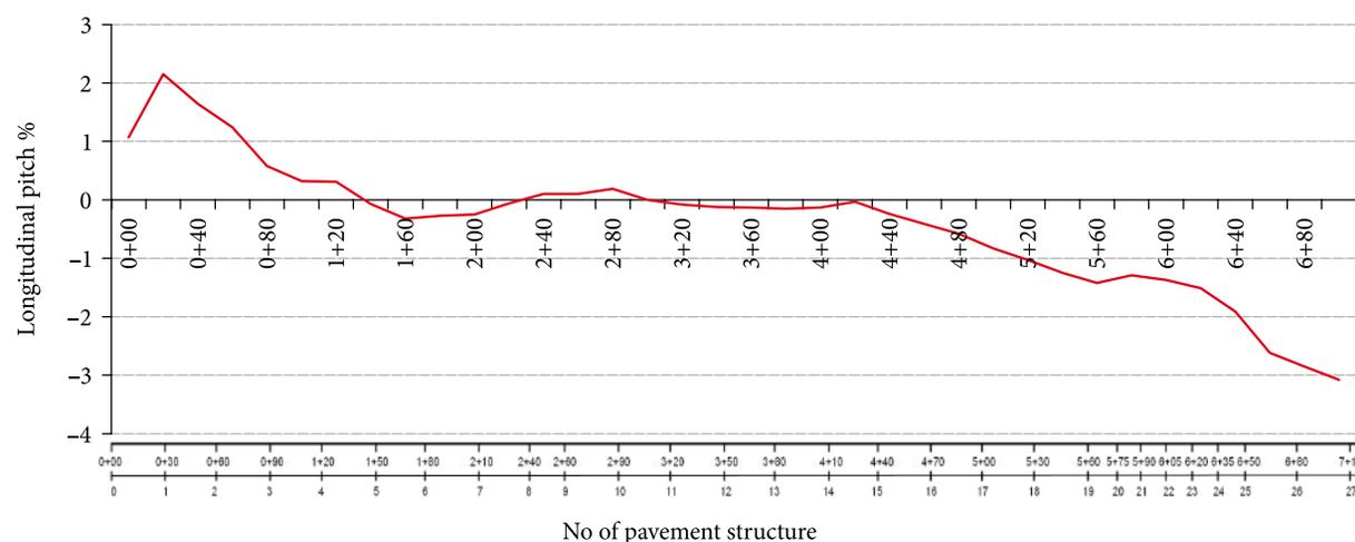
Fig. 7. The chart of longitudinal cross falls of a test road sections
