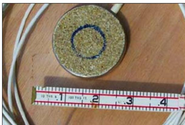
Fig. 3. Stress transducers installed in experimental pavement structures
