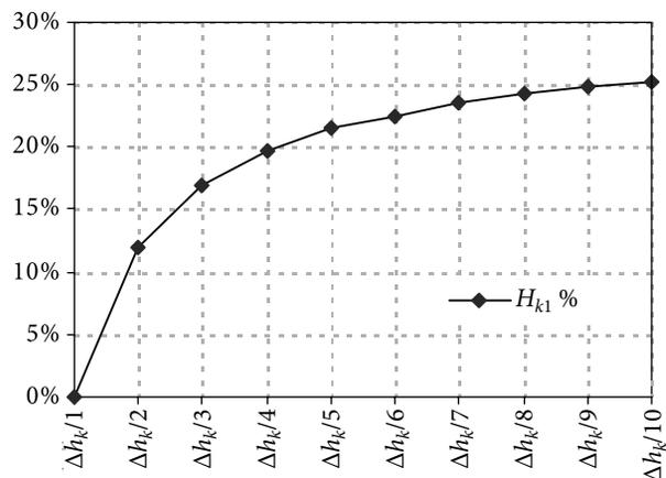
Fig. 6. Relation of horizontal force  $H_{k1}$  relative magnitude vs horizontal displacement  $\Delta h_k$
