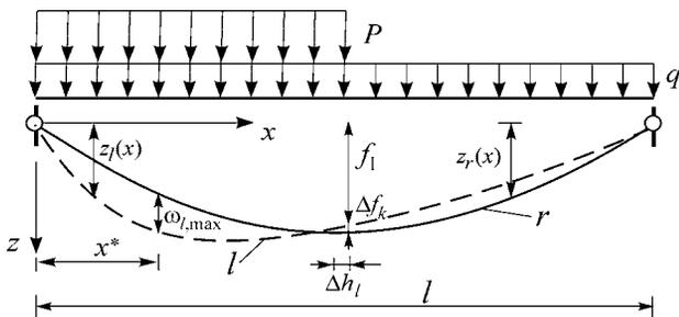
Fig. 1. Deformed scheme of asymmetrically loaded cable
