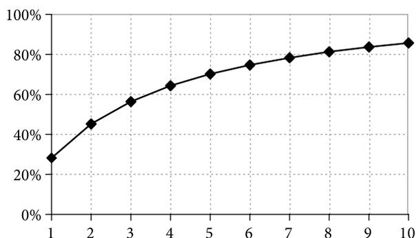
Fig. 2. Relative difference in % of cable right and left parts max displacements vs loads ratio  $\gamma$
