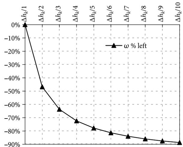
Fig. 5. The cable left part kinematic displacement  $\omega_{l,max}$  vs horizontal displacement  $\Delta h_k$
