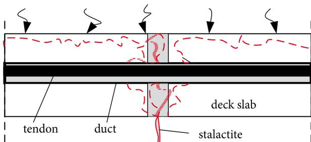
**Fig. 4.** The effect of leaching on the underside of concrete deck of box girder due to leakage of epoxy joint
