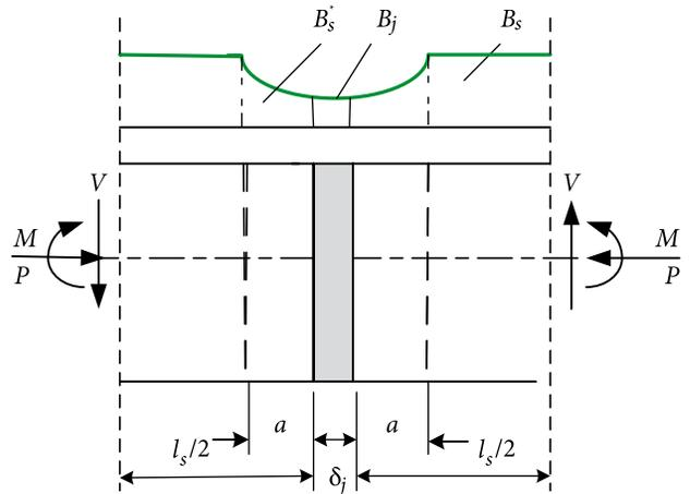
Fig. 3. Idealized model for segmental joint and definition of the joint rigidity problem to be solved
