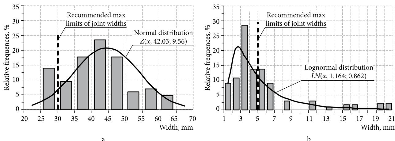
Fig. 2. The distribution of the joint widths for cast-in-place (a) and epoxy (b) joints
