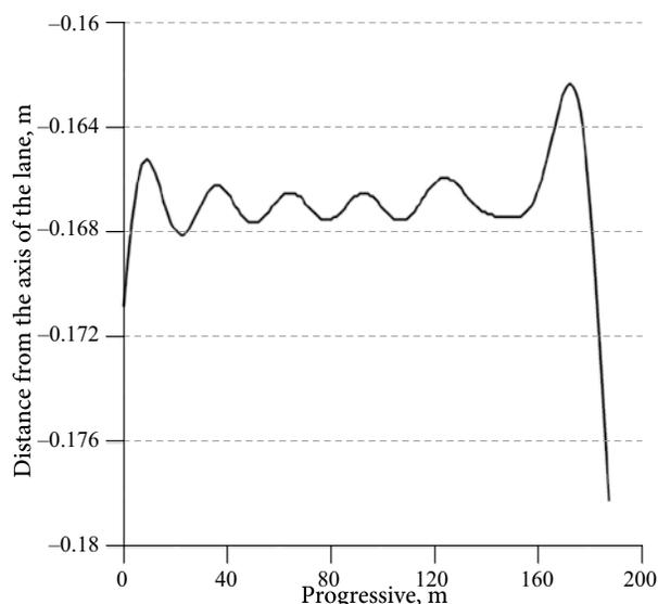
Fig. 9. Position of the vehicle respect to the centre line of the lane to verify the presence of underload
