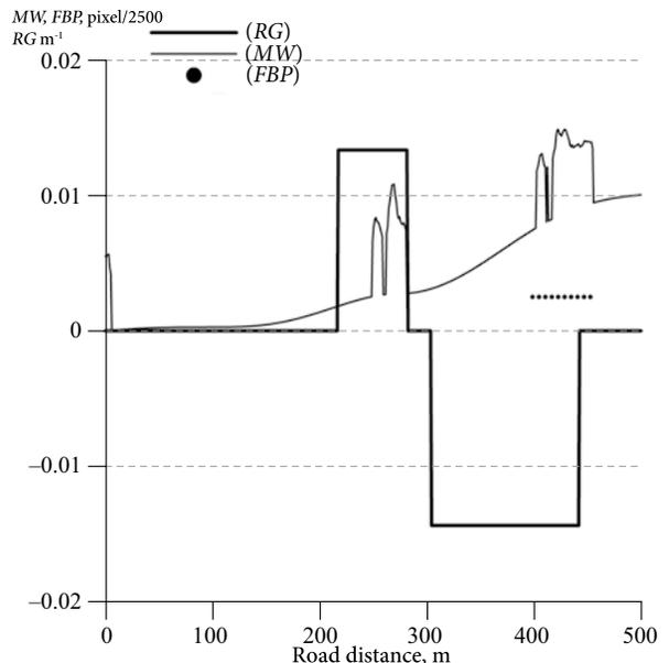
Fig. 5. Relationship between *MW*, deduced from the sum of *E* and *VLI*; in the section from 400 to 460 m there is an activity on the foot/break pedal represents an overload situation
