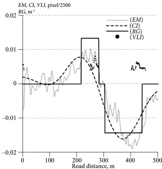
**Fig. 6.** Relationship between CI function of the sample and EM and VLI for a specific driver (the ordinates in pixel of EM, CI and VLI were scaled for 2500 to represent also the curvature diagram (RG) in the same graphic; the data concern the road distance from 0 to 500 m)
