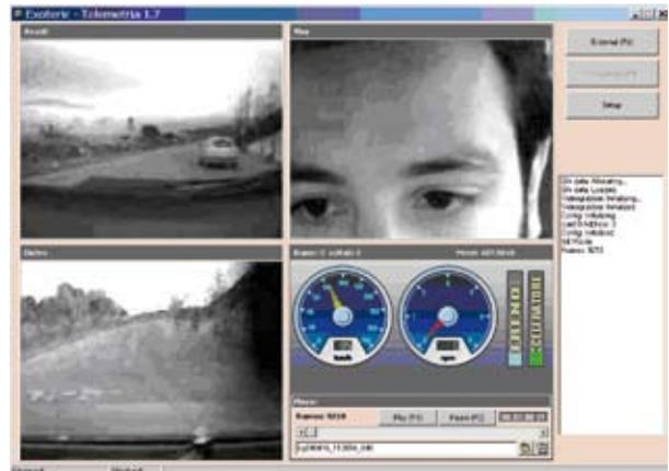
Fig. 1. Graphic interface of the 3 video cameras and the telemetry in real time
