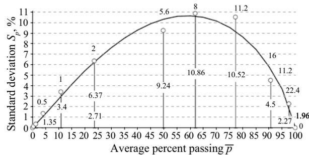
Fig. 4. Correlation between the parameters of RAP-3 non-extracted granules gradation variation ( $s_p$ ) and position ( $\bar{p}$ )
