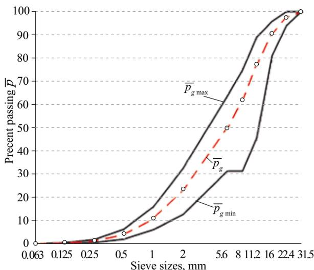
Fig. 2. Gradation of non-extracted granules of milled AP being recycled (RAP-3) (sample size  $n = 15$ )
