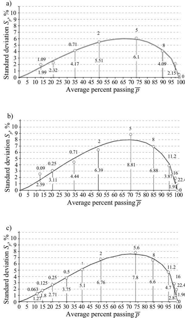
Fig. 3. Correlation between the parameters of milled RAP aggregate gradation variation ( $s_p$ ) and position ( $\bar{p}$ ) determined for the following samples: a – RAP-1; b – RAP-2, c – RAP-3
