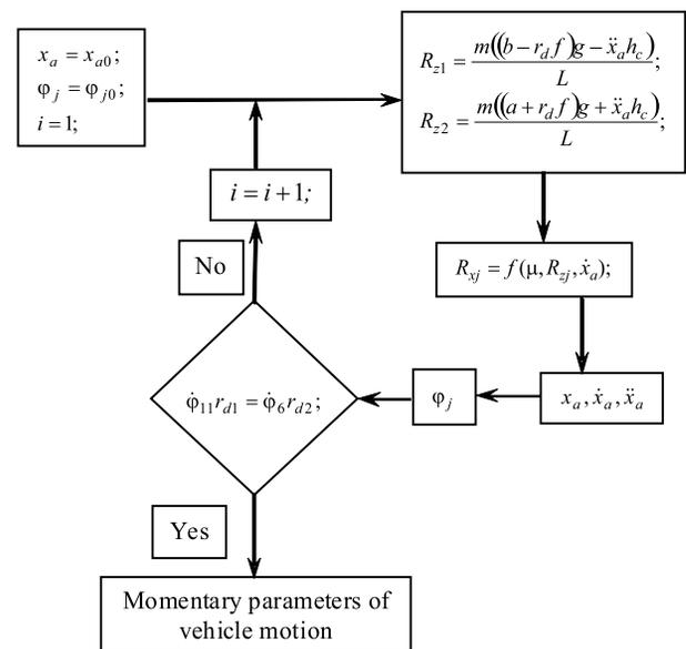
Fig. 4. Algorithm describing the tyre and road interaction (Starevičius 2007)
