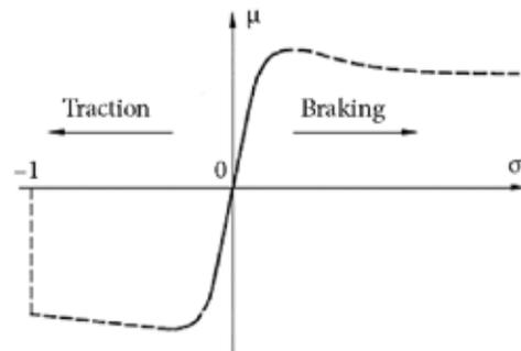
**Fig. 3.** Dependency of  $\mu$  on sliding in traction and braking regimes
