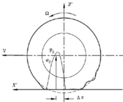
**Fig. 1.** Distribution of the normal pressure in the tyre-road contact zone
