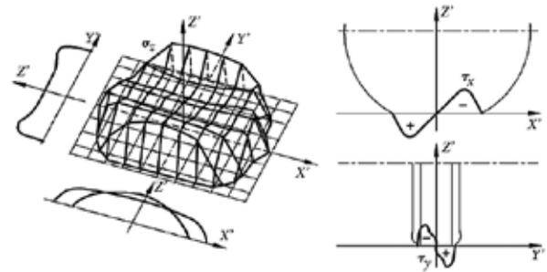
**Fig. 2.** Distribution of pressure components in the tyre-road contact zone
