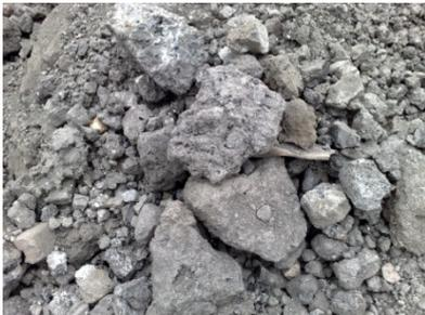
Fig. 1. Unfractionated BOF slag aggregate
