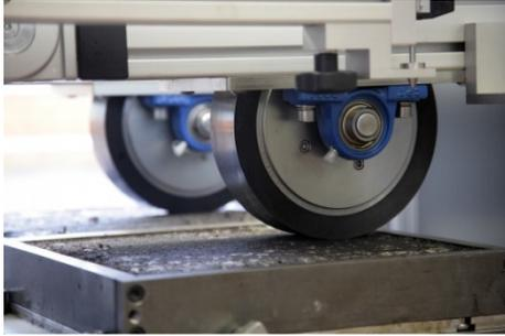
Fig. 3. Test equipment for wheel tracking test
